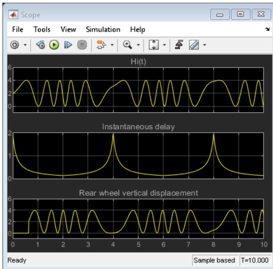
Figure 2: Vertical displacement of the wheels.
